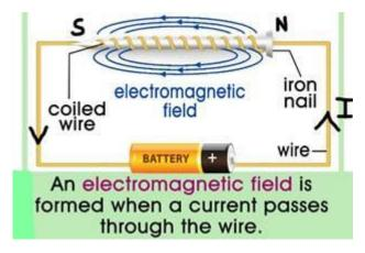
Q.4. Describe an activity to demonstrate the direction of the magnetic field generated around a current carrying conductor.
