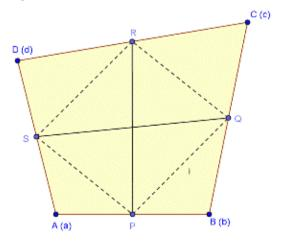
Let ABCD be a quadrilateral and P,Q,R,S be the mid points of sides AB, BC, CD and DA respectively.
